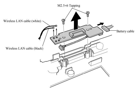
Figure 4-37 Removing the power board
